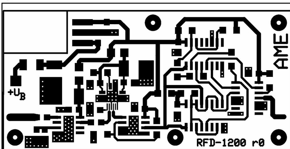
Fig 2: Printed circuit board layout for 12GHz divide by 1000 prescaler.
