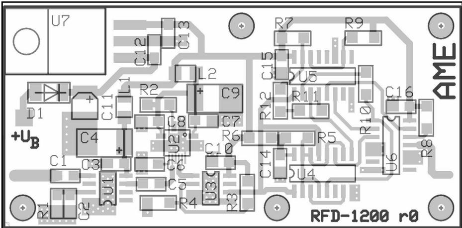
**Fig 3: Component layout for 12GHz divide by 1000 prescaler.**
