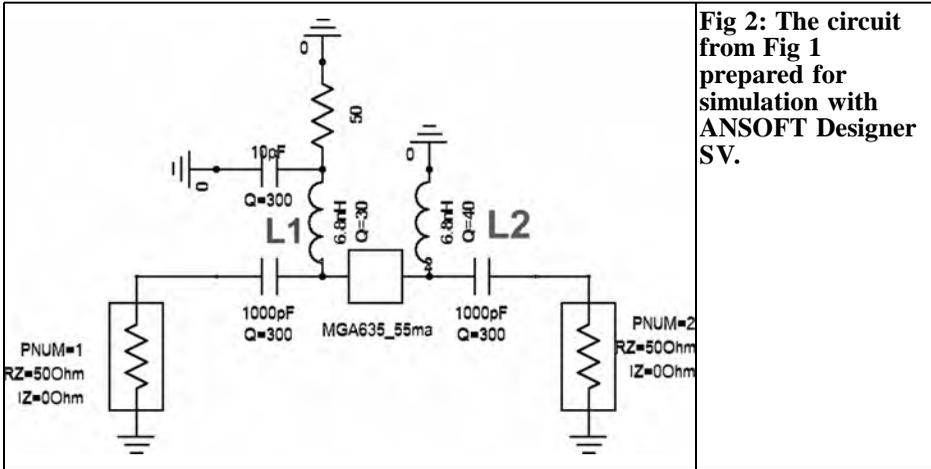
**Fig 2: The circuit from Fig 1 prepared for simulation with ANSOFT Designer SV.**
