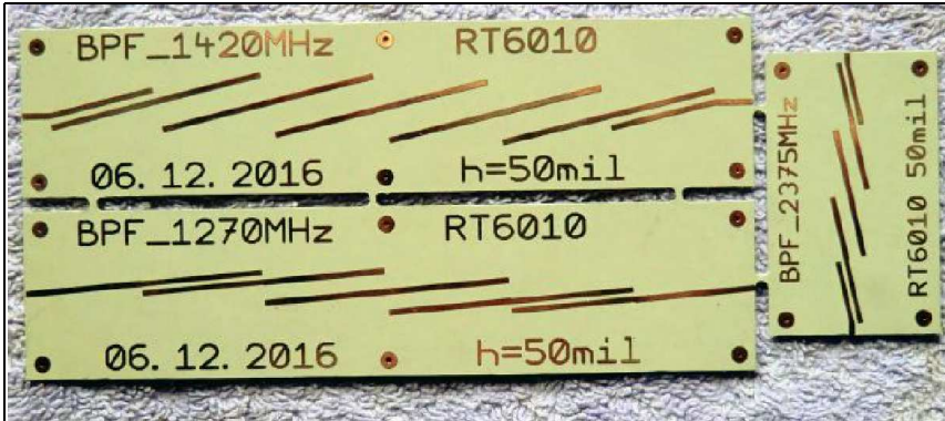
Fig 31: This is the "benefit" of professional board production (here Teflon material). Because of the high material and preparation costs you try to produce as many circuits as possible.
